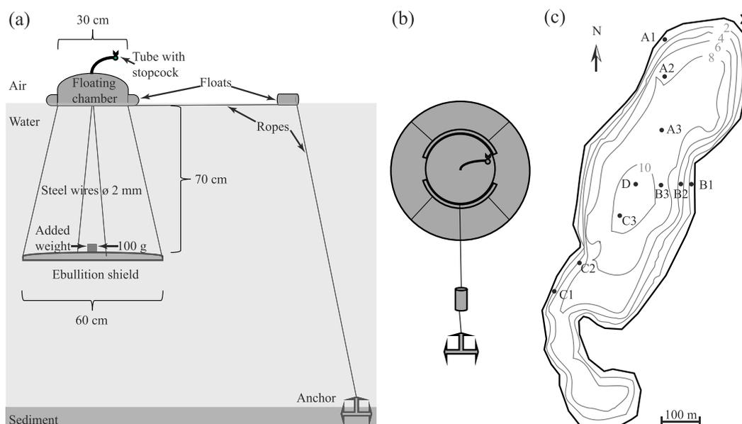
**Figure 1.** (a) Schematic representation of our adaptations to the floating chamber design presented by *Cole et al.* [2010]. (b) Top view of our shielded floating chamber setup. (c) Bathymetric map of Lake Gerzensee showing the locations of the sampling stations. The numbers indicate the depths of the isobaths, and the cross marks the location of the weather station.
